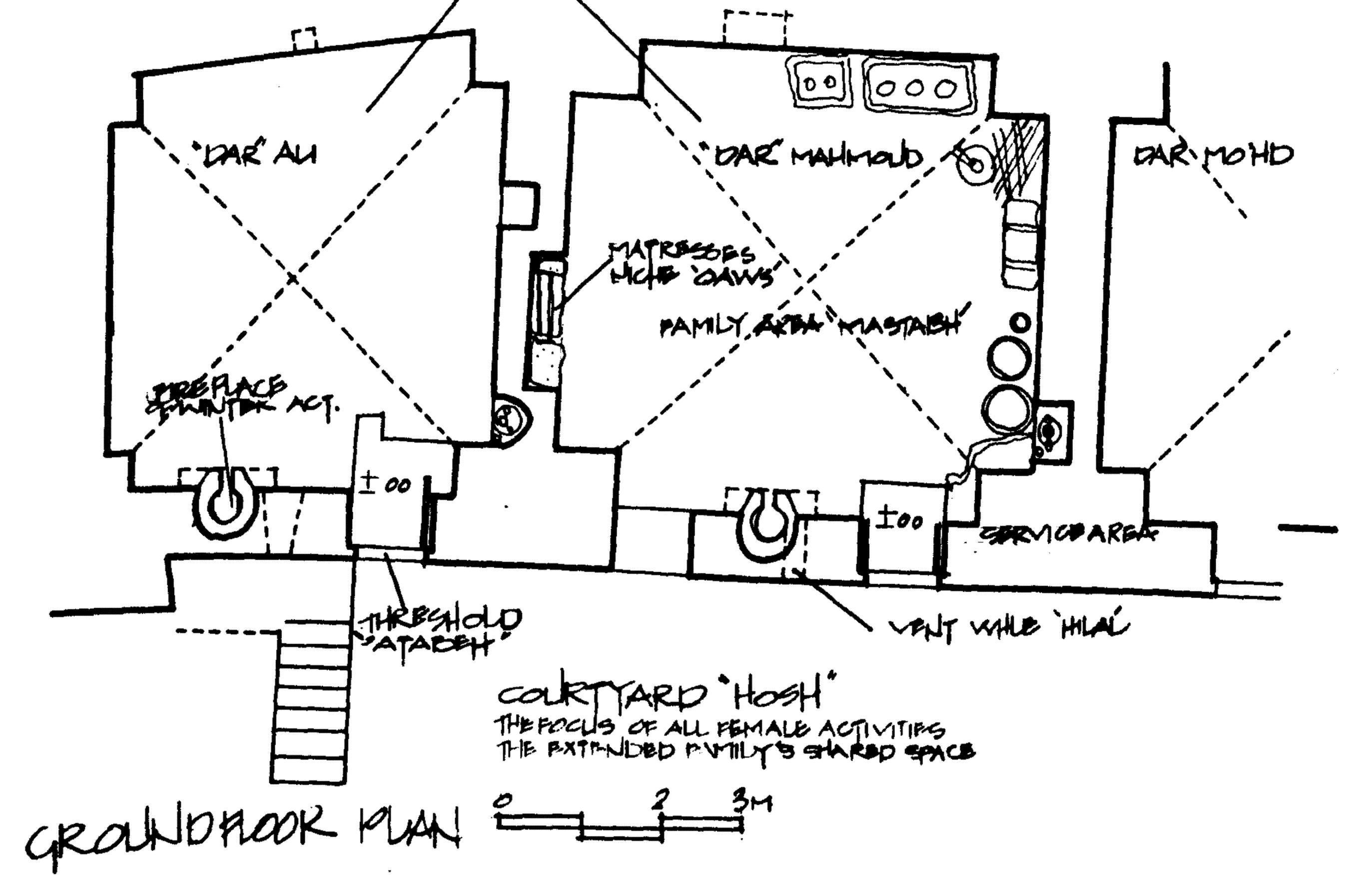
Fig. 4.21: Plan showing the interior layout of two adjacent houses
